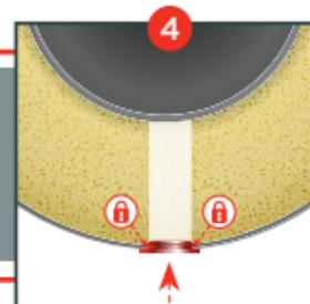
**STEP 4** Install silicone grommet into the cut out hole in the cladding.
