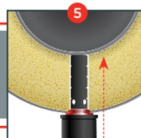
**STEP 5** Insert Water Indicator into silicone grommet and push fully into place.
