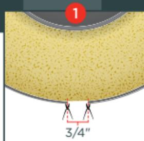
**STEP 1** Cut/drill a 3/4" hole in the desired location in cladding using tin snips or a hole saw. *ensure the hole saw only penetrates the cladding*
