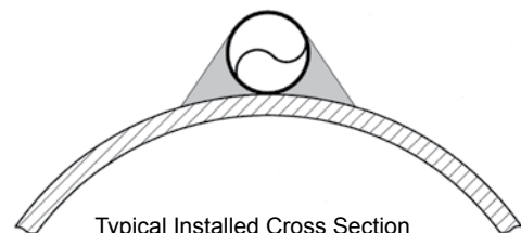
Typical Installed Cross Section (Fillet application)
