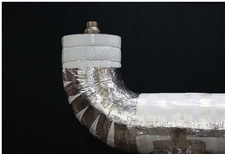
Figure 20: Butyl tape to form secondary vapor barrier.
