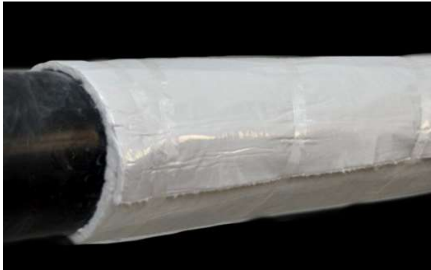
Figure 13: Single layer with overlapping longitudinal joint. Circumferential tape overlapping 50%.
