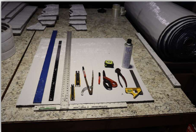
Figure 2: Recommended cutting and measuring tools.
