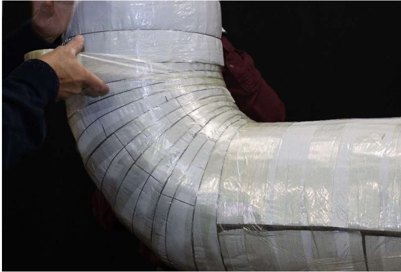
Figure 19: Outer layer gored joints secured with filament tape.
