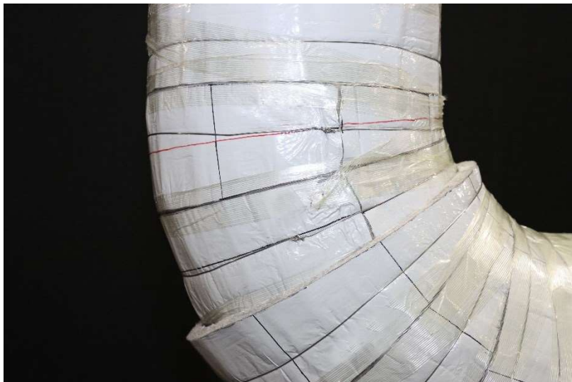
Figure 18: Staggered second layer of elbow gores.
