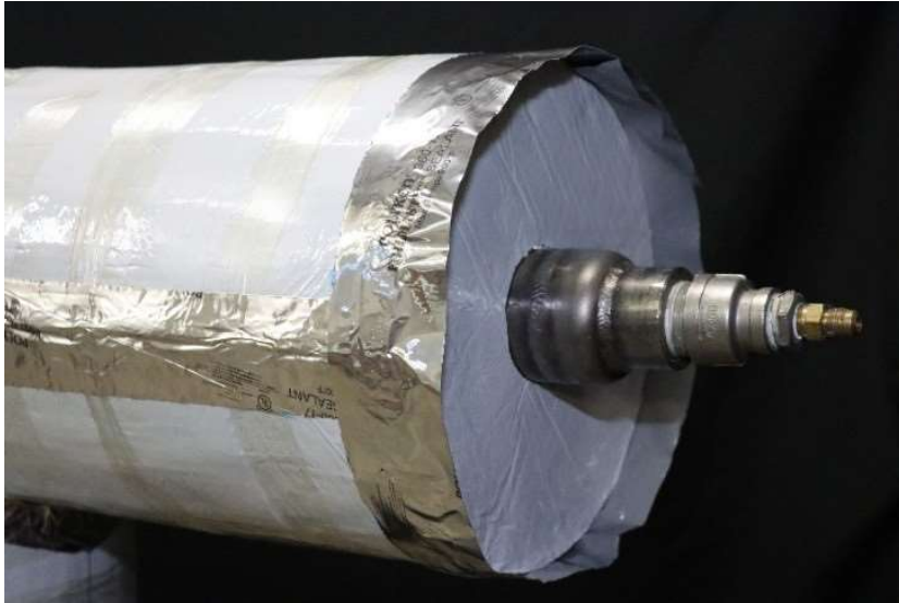
Figure 35: Butyl based aluminum tape over secondary vapor barrier.
