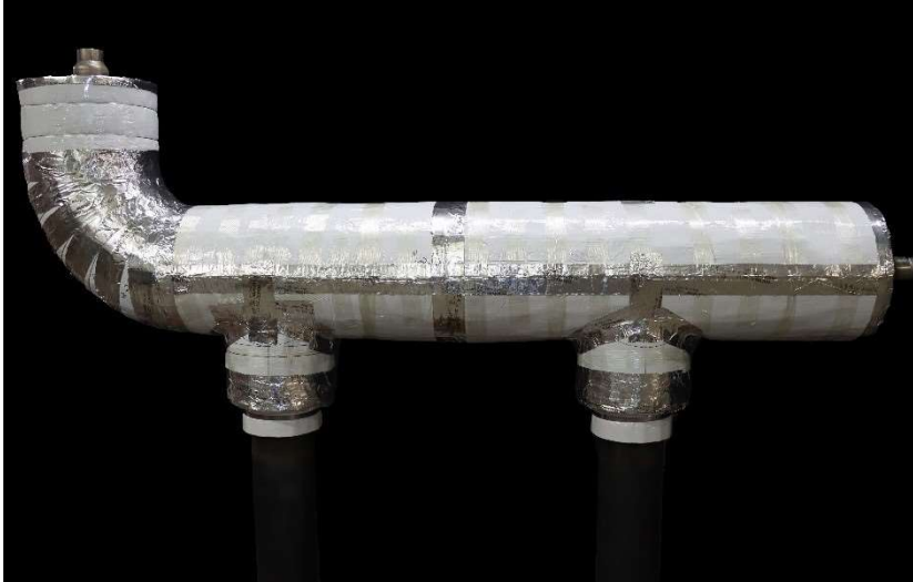
Figure 4: Butyl-backed aluminum tape applied over secondary vapor barrier.
