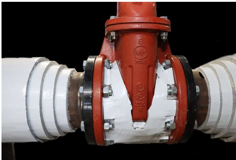
Figure 40: Insulation termination distance from flange to allow bolt removal space.
